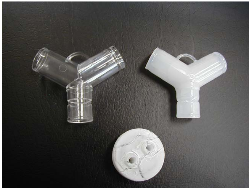
Figure 5 shows premature failure of a part that was exposed to aggressive chemicals.
